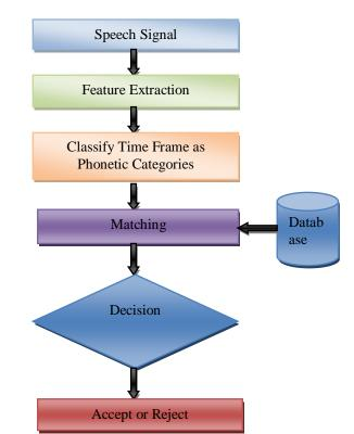
Fig.1: Flow Diagram of Speech Recognition System
